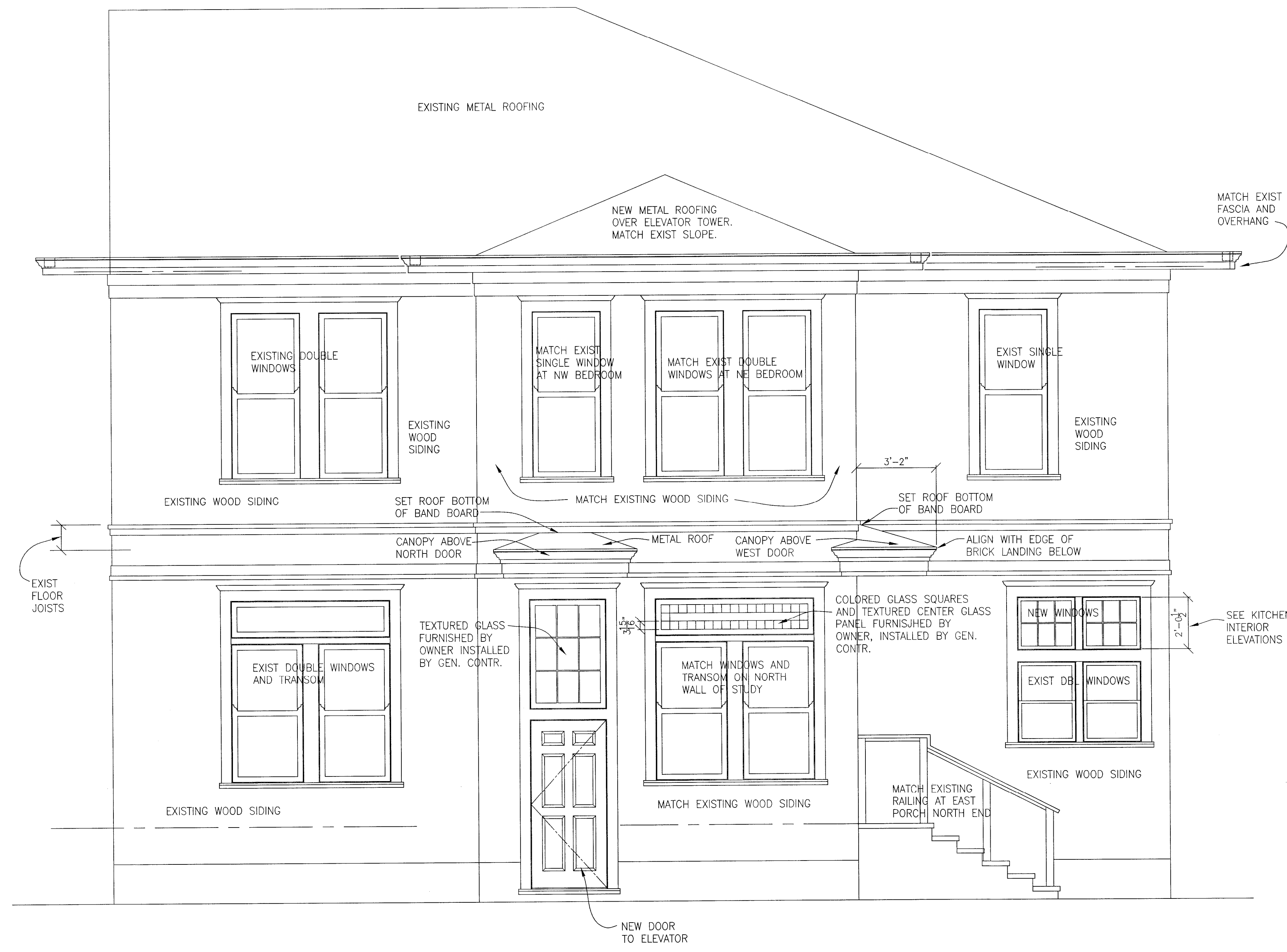
EXTERIOR ELEVATION - NORTH SCALE 3/8" = 1'-0"
