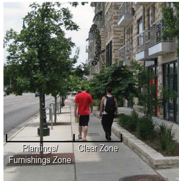
Figures 8-1 Illustrations delineating the Streetscape Zone elements
